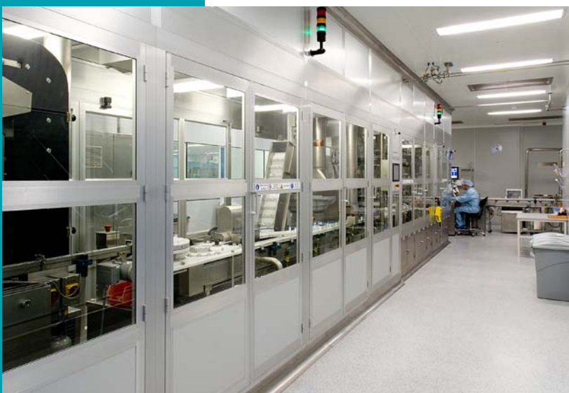
IVAX automated nebulizer filling line
